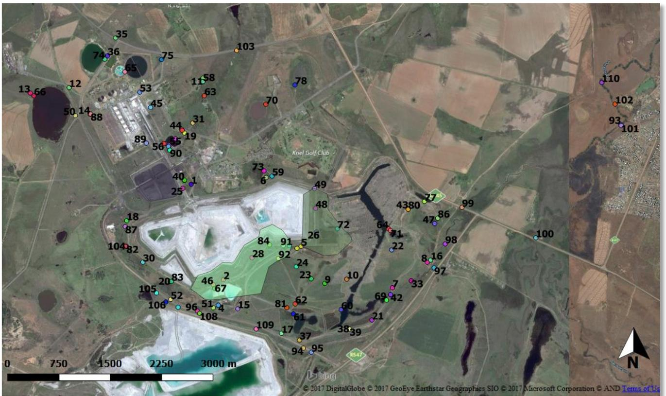
Figure 10-1 | Existing monitoring boreholes around the Kriel Ash Disposal Facility.
